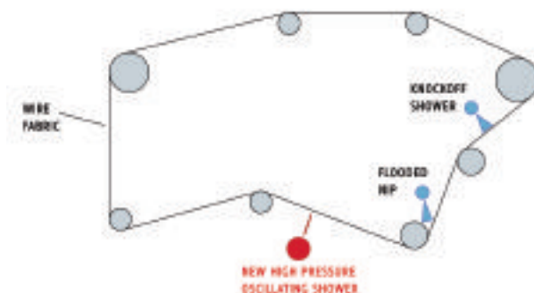
Figure 3: Schematic of forming fabric section at Simpson-Clough Mill
