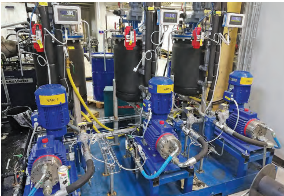
Three P500 models replaced six piston pumps for spraying an adhesive colorant and substantially reduced maintenance costs.
