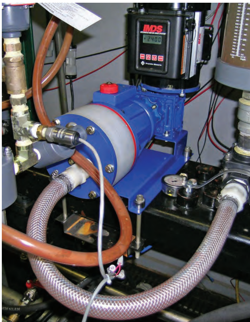
P400 used with several metering accessories in a testing laboratory.
