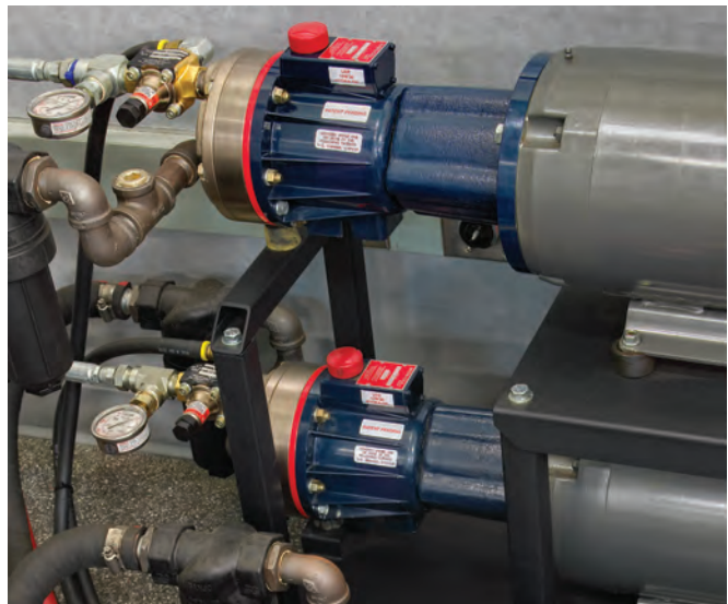
Hydra-Cell pumps can also be mounted externally to the machine tool system.
