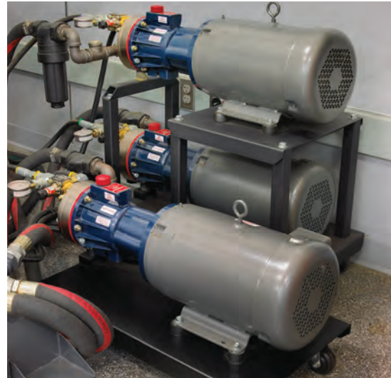
Three Hydra-Cell model D10 pumps deliver high-pressure coolant for a turret-type, multi-tasking boring machine with 16 tool stations for bar work and 12 tool stations for chuck work.
