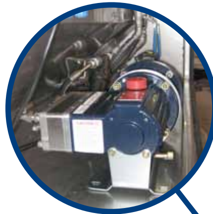
Explosive Injection Charging liquid explosives into blast holes
