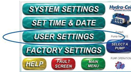
Enter Model #, Motor RPM, and System Pressure for your pump.
