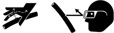
Check tubes, hoses and fittings for damage and leakage. Never use bare skin to check for leaks. Equipment tubes and hoses must be properly routed and have adequate support and secure clamps. Repair any leakage problems by adjusting or replacing parts as indicated upon inspection.
